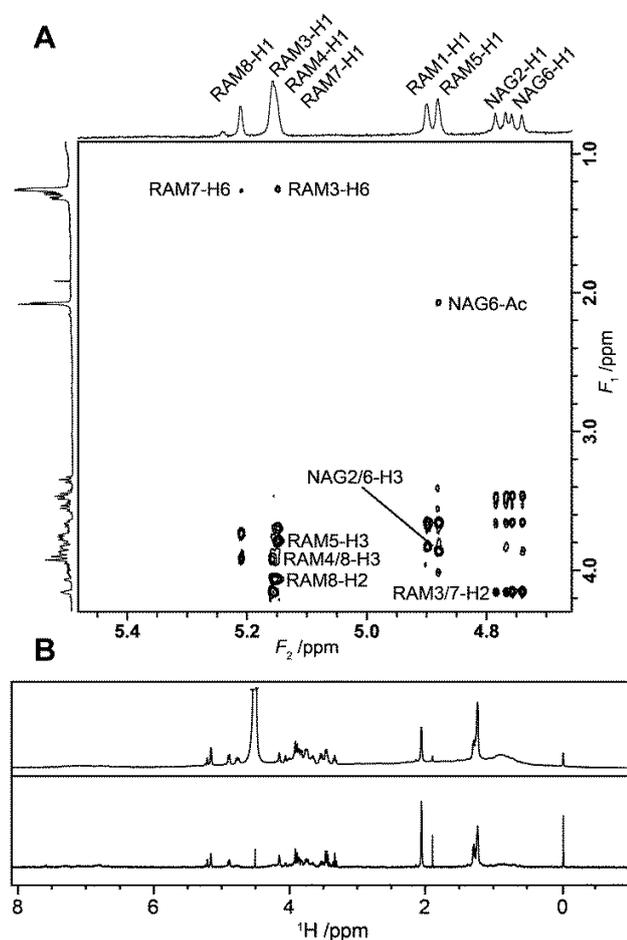
Figure 2. Figure caption. (A)  $^1H, ^1H$ -trNOESY spectrum with selected inter-glycosidic cross-peaks annotated. (B)  $^1H$  NMR spectrum (top) and a STD spectrum (bottom) of Sf6TSP with the octasaccharide in  $D_2O$ . The irradiation frequency in the STD experiment was set to 7 ppm, and the saturation time was 2 s.
