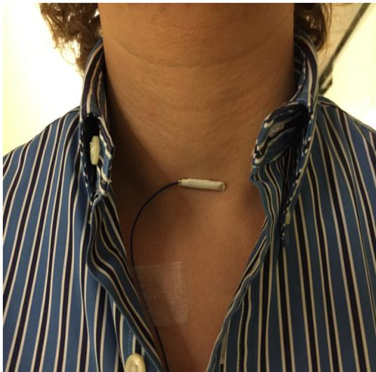
Figure 2. Throat microphone attached to a speaker's neck.
