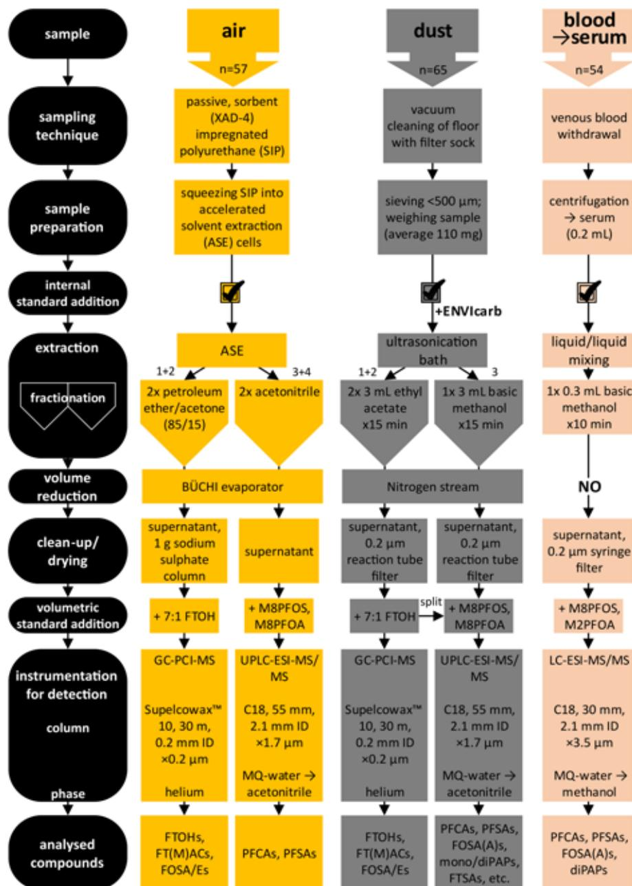
Figure 4: Workflow scheme on sample treatment, extraction and analysis.
