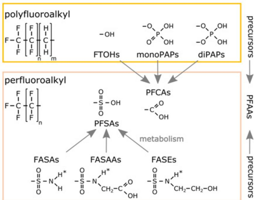
**Figure 1:** Generic chemical structures of PFASs and their division into subclasses relevant for this thesis, including metabolic routes to PFCAs or PFSAs from various precursors; Note for FASAs/AAs/Es: replacing the  $-\text{H}$  marked with an asterisk (\*) by  $-\text{CH}_3$  (methyl) or  $-\text{CH}_2-\text{CH}_3$  (ethyl) leads to name prefixes “Me-” or “Et-”, respectively.
