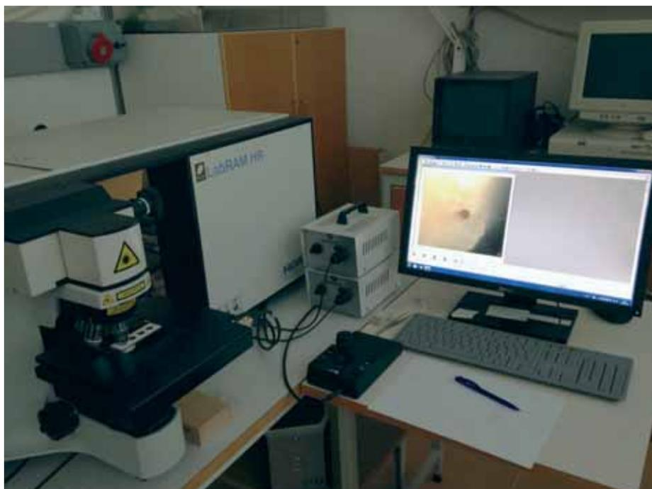
**Figure 14.** Raman instrument showing on the computer screen (right) a brownish spot growing on foraminiferal test calcite.
