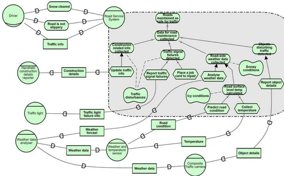
Fig. 2. i\* Strategic Rational Model for the road maintenance service, with identified data resource dependencies to digital sources for required service capabilities (tasks).
