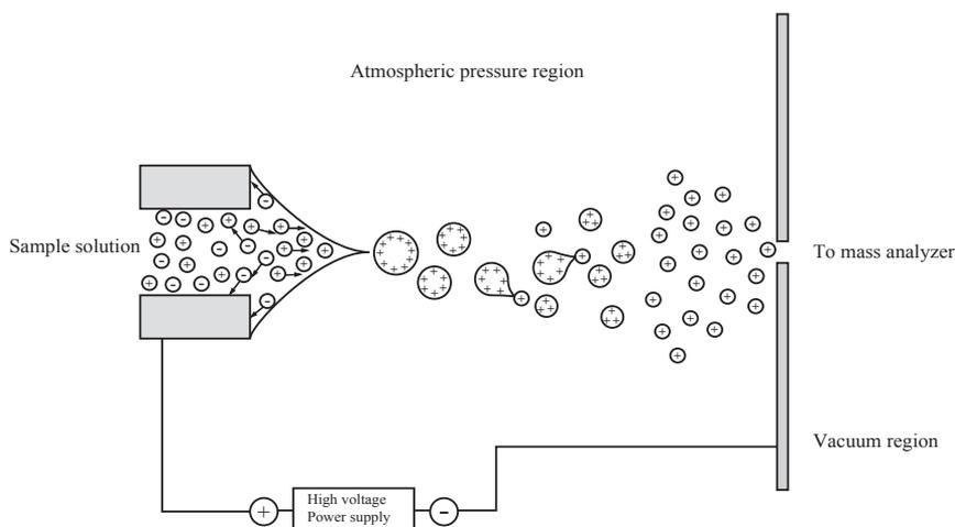
**Figure 12.** Schematic representation of the ESI process, in this case in positive ion mode.
