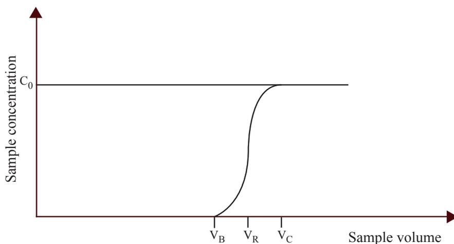
**Figure 2.** A theoretical representation of a typical breakthrough curve.  $V_B$  is the breakthrough volume,  $V_R$  is the chromatographic elution volume and  $V_C$  corresponds to the sample volume at which the capacity of the sorbent is saturated. At  $V_C$  the concentration of the analyte entering the sampling device is the same as the concentration of the analyte exiting the device,  $C_0$ .
