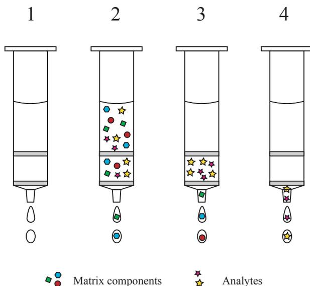
**Figure 3.** The four steps of the SPE process, conditioning (1), sample application (2), washing (3) and elution (4).
