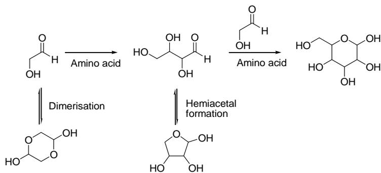
**Scheme 3:2.** The possible cyclisations that can occur if performing the reaction with unprotected alcohol functionality.
