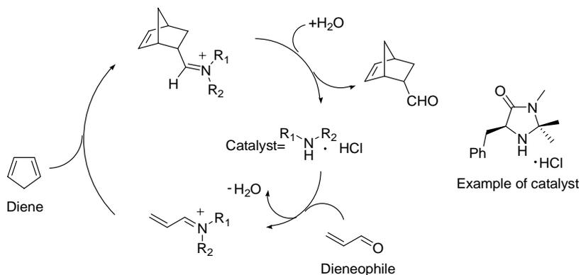
**Scheme 1:2.** Diels Alder reaction mediated by an organocatalyst that conducts the reaction via formation of an iminium salt with the dieneophile.
