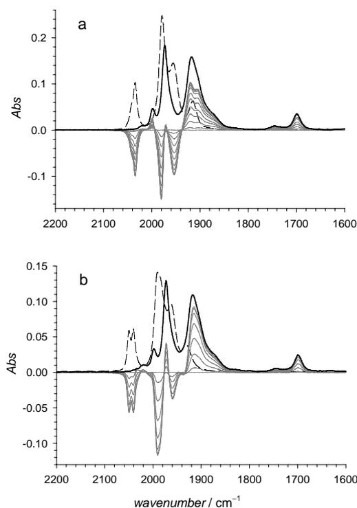
**Figure 14.** IR spectrum of complex **19** (a) and **20** (b) before (dashed line) and after (solid line) the electrochemical reduction at  $-1.98$  and  $-1.78$  V, respectively. Grey traces are difference spectra recorded during the course of the electrolysis.
