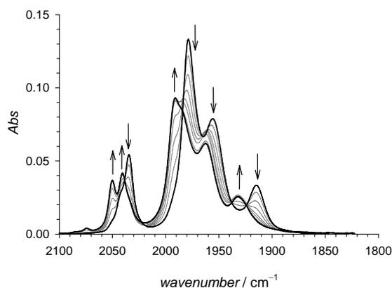
**Figure 12.** The spectral changes in the carbonyl region of the IR spectrum upon the transformation from **19** to **20**.
