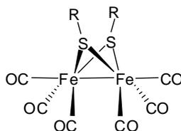
**Figure 10.** Complexes of the general formula  $(\mu\text{-RS})_2\text{Fe}_2(\text{CO})_6$ .
