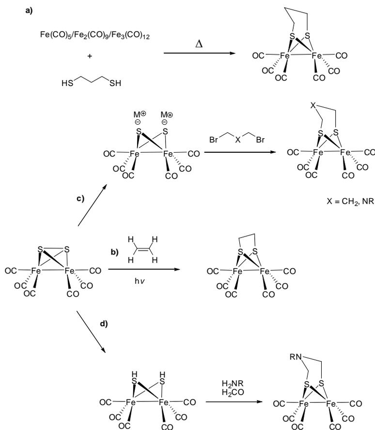
**Scheme 9.** Synthetic methods to obtain complexes of the general formula  $(\mu\text{-}(\text{R})\text{S})_2\text{Fe}_2(\text{CO})_6$ .
