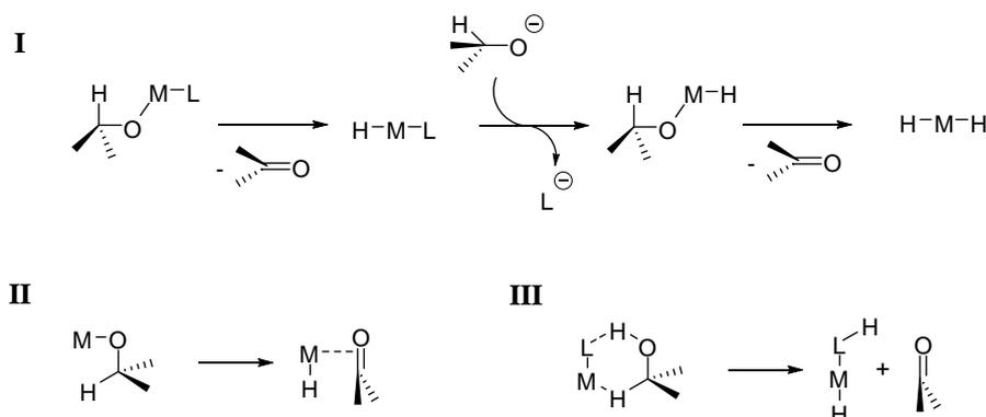
**Scheme 2.** The di-hydride (I), the mono-hydride inner-sphere (II) and the mono-hydride outer-sphere (III) mechanisms.
