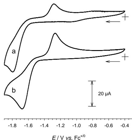
**Figure 13.** The cyclic voltammogram (100 mV/s) of: a) **19** obtained in the presence of excess *n*-propylamine and b) **20** in MeCN solution.
