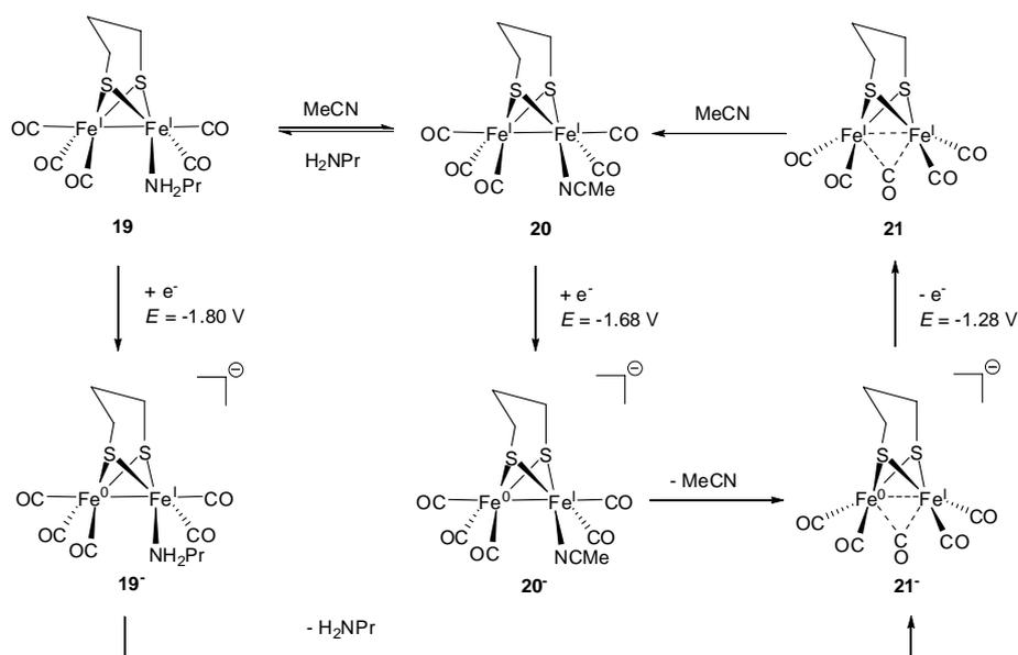
**Scheme 13.** A proposed cycle for the electrochemical transformations of complex **19**.
