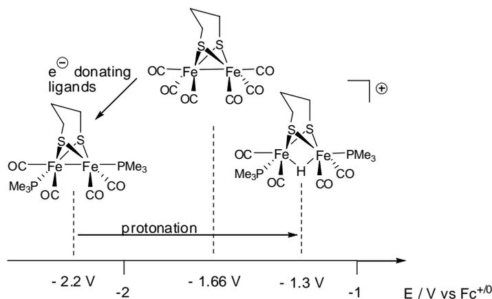
**Scheme 10.** Introduction of electron donating ligands that enable subsequent protonation and their effect on the reduction potential of the complexes.
