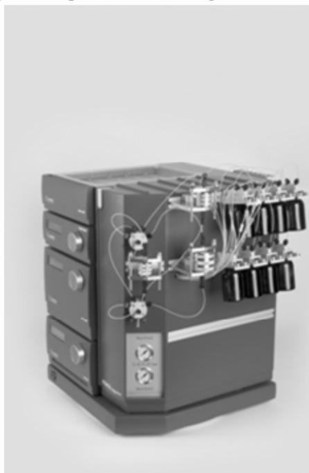
**Figure 3.1:** Oligonucleotide synthesis was performed with an ÄKTA oligopilot synthesizer.
