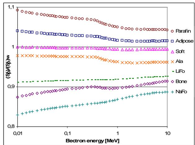
Fig13b Log-Lin plot of mass collision stopping power coefficients as a function of electron energy.
