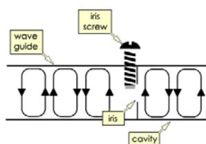
Fig3a The iris of the waveguide is adjusted to achieve standing waves in the cavity and no reflection back to the waveguide.
