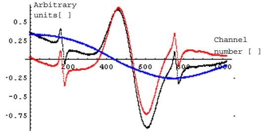
Fig15d BP-filtering of the perturbed spectrum of LiFo resulting in heavy distortion due to insufficient spectral width compared to peak width of LiFo.
