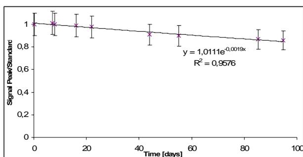
Fig21a Three month fading of ESR-signal for LiFo, normalised to  $Mn^{2+}(MgO)$  and the initial value.
