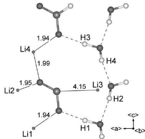
Fig8b Crystal structure around a radical in LiFo
