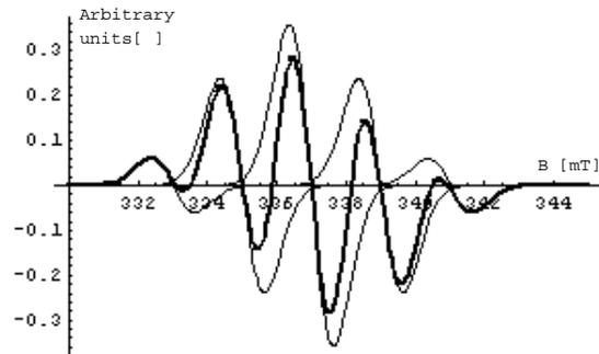
Fig5a Derivative spectrum (first harmonic output) of the absorption peaks to the left.
