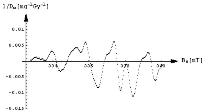
Fig14c Spectrum of ZnLa at  $P=2$  mW,  $-B_m=0.37$  mT
