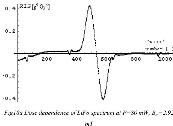
Fig18a Dose dependence of LiFo spectrum at  $P=80$  mW,  $B_m=2.92$
