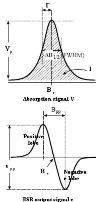
Fig4b Principal shape of spectral peaks and abbreviations used to describe spectral characteristics. (After Truitt 2004)
