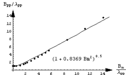
Fig6b Fitting of model function for  $B_{pp}$  to the data of Smith.
