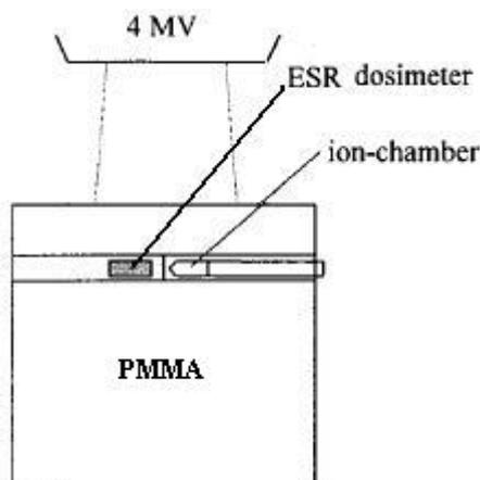
*Fig9 Experimental set-up during clinical irradiation of pellets (After Olsson & Bergstrand 2001).*
