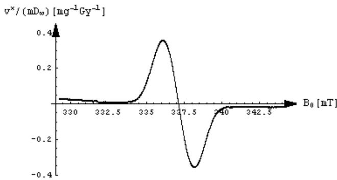
Fig14a Spectrum of LiFo at  $P=80$  mW,  $B_m=2.92$  mT
