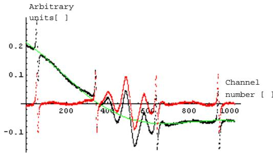
Fig15a Conventional baseline correction, of the perturbed spectrum of Ala, by subtracting a baseline fitted 6th order polynomial.
