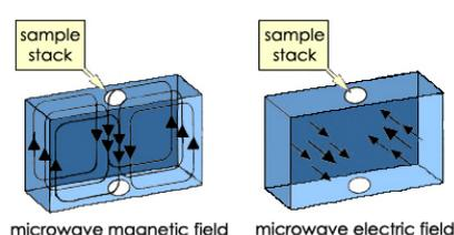
Fig3b The magnetic and electric field due to standing waves in the cavity. The stack for the sample test tube is indicated
