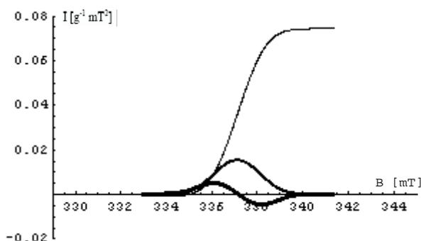
Fig20a Output spectrum (thick graph), integral resembling the absorption spectrum and double integral (thin graph) for LiFo
