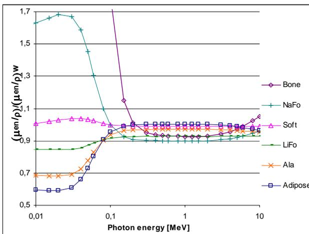
Fig13a Log-Lin plot of mass energy-absorption coefficients as a function of photon energy
