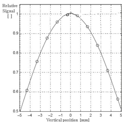
Fig 11a Signal deviation as a function of vertical displacement in the cavity. (after Anton 2005)
