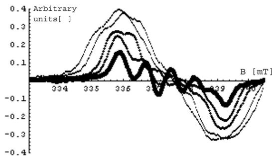
Fig16a Modulation broadening effect to hfs-structure of NaFo.
