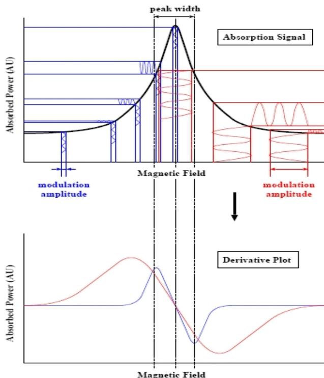
Fig4a Moderate modulation (left in upper part), overmodulation (right in upper part) and the resulting output spectra (lower part). (From Truitt 2004)
