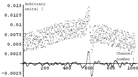
Fig 12a Simulation of a spectral peak, afflicted with heavy perturbation of a broad signal and high frequency noise (points) and the filtrated spectrum (line).
