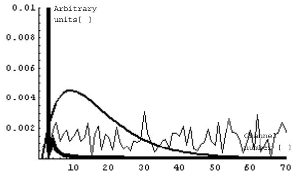
Fig12b Fourier transform of the broad signal (thick line), the spectral peak and the noise (thin line). The frequency limits of the BP-filter, of the proposed method, would be channel 6 & 30.
