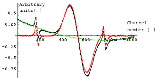
Fig15c Same as 15a but with LiFo and half the scan width. The fitting is more difficult because only limited parts of the spectrum can be used for the polynomial fit.
