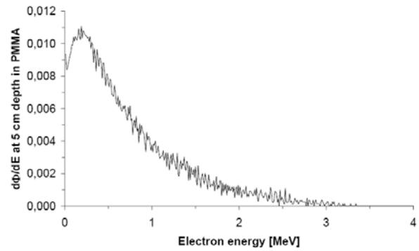
Fig10b Electron fluence at the reference depth in the phantom irradiated with 4MV photons. (After Olsson & Bergstrand 2001).
