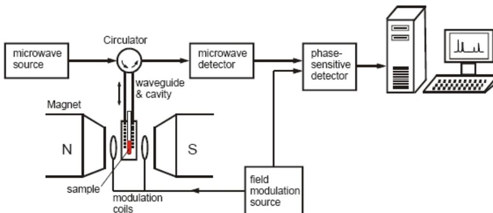
Fig 2 Schematic block diagram of the ESR-CW spectrometer (From Jeschke 2003)
