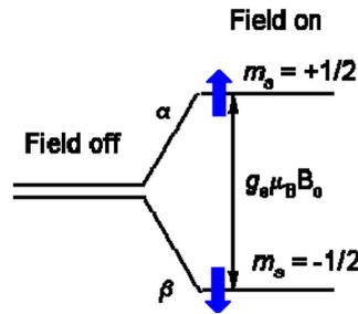
Fig1 Paramagnetic states of an unpaired electron and their energy.
