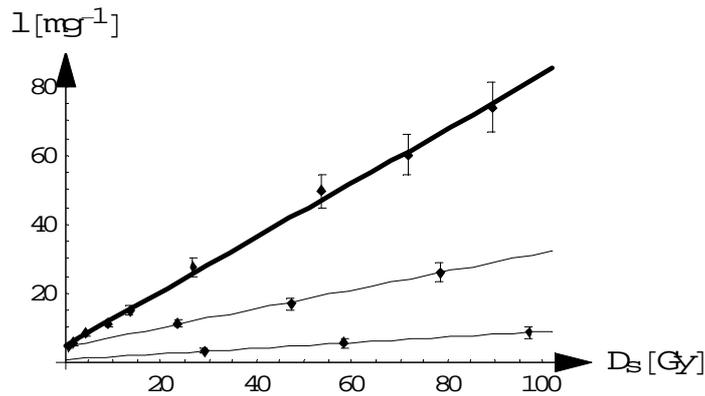
Fig19a. Dose response in water equivalent phantom for LiFo (thick graph), NaFo and Ala (thin graph).
