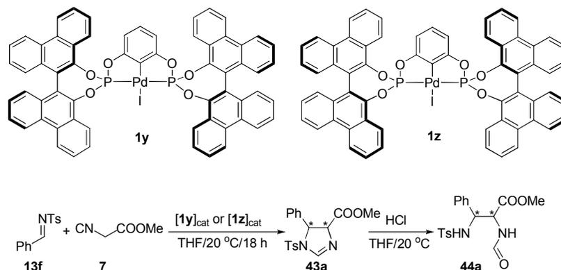
**Scheme 17.** Asymmetric condensation of sulfonylimine **13f** and isocyanoacetate **7**.
