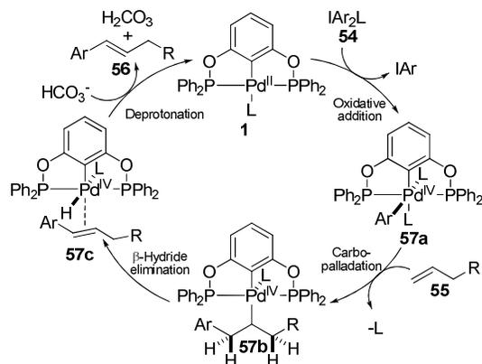
**Scheme 23.** Proposed Pd(II)/Pd(IV) catalytic cycle.
