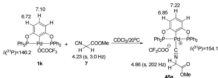
**Scheme 15.** Change of NMR shifts (ppm) in the stoichiometric reaction of **1k** and **7**.
