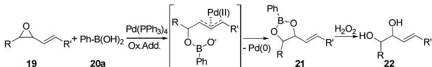
**Scheme 6.** Pd(0) catalyzed C-O coupling with arylboronic acids and vinyl epoxides.
