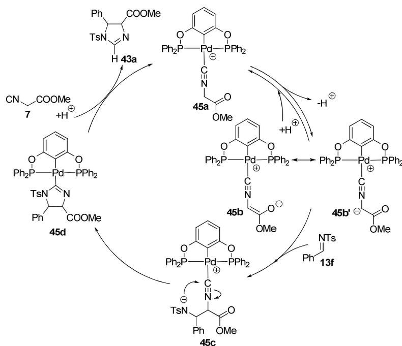
**Scheme 16.** Plausible catalytic cycle based on the mechanistic studies.
