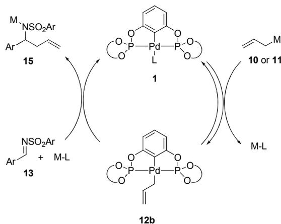
**Scheme 13.** Proposed catalytic cycle for the allylation of sulfonylimines.
