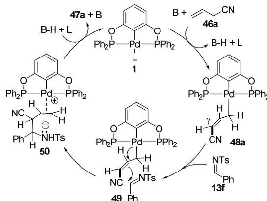
**Scheme 19.** Mechanistic proposal for the catalyzed allylation of sulfonylimines.
