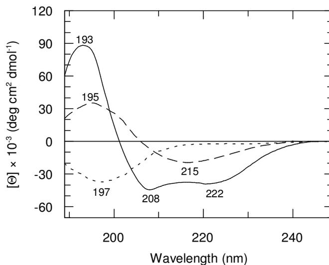
**Figure 11.** Shapes of CD spectra measured for various secondary structures;  $\alpha$ -helix (black line),  $\beta$ -sheet (long dashes) and random coil (short dashes) (126).
