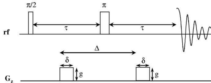
**Figure 8.** Pulse sequence for translational diffusion NMR. The transverse magnetization, generated by a  $90^\circ$  pulse, is first subjected to a gradient of strength  $g$  and duration  $\delta$ . During the delay  $\Delta$  a  $180^\circ$  pulse is applied and before acquisition there is another gradient, identical to the first one (117).
