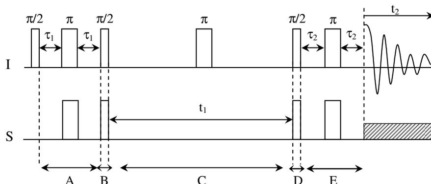
**Figure 7.** Pulse sequence of the HSQC experiment. Period A and B constitute an INEPT step during which proton magnetization is transferred to a low gyromagnetic ratio nucleus like  $^{13}\text{C}$  or  $^{15}\text{N}$ . During C the S spin magnetization evolves and is subsequently transferred back to the I spin during D and E that constitute a reversed INEPT step. In the acquisition period the S spin is decoupled (dashed rectangular box) to avoid heteronuclear splitting of the peaks (113).
