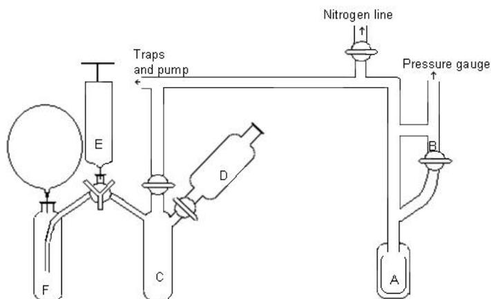
**Figure 4.1.** The vacuum manifold for transfer of  $^{35}\text{S}$ -sulfur dioxide into reaction vessel. A – vial with sulfuric acid, B – stopcock for controlled addition of granular copper, C – cold trap, D - oil funnel, E – syringe for controlled addition of sulfur dioxide, F – reaction vessel. The manifold was designed in house and manufactured for the  $^{35}\text{S}$ -PFSA syntheses.
