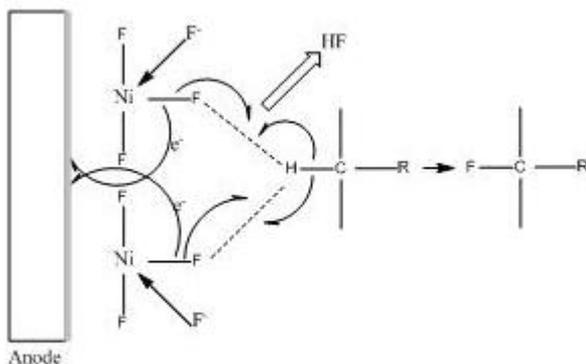
**Figure 2.1** Proposed ECF process. The substrate is oxidatively fluorinated at the anode surface [54].
