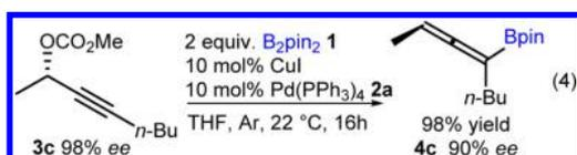
Pd(PPh<sub>3</sub>)<sub>4</sub> and CuI catalysts at room temperature, chiral allenyl-Bpin **4c** was obtained. The stereochemical outcome of this reaction and the procedure by Ito and Sawamura (eq 1)<sup>2a</sup> are identical.
