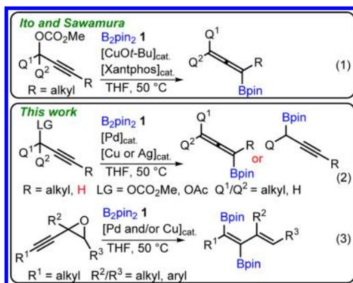
synthetic approaches to a large variety of allenyl boronates.<sup>1f,g,2b</sup> This procedure (eq 1) usually requires use of freshly sublimated  $CuOt$ -Bu to give high yields. In addition, terminal alkynes could not be used as substrates, probably because of the easy deprotonation by the  $CuOt$ -Bu catalyst.
