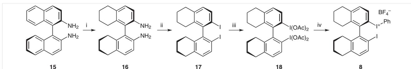
**Scheme 5** Synthesis of diaryliodonium salt **8**. Reagents and conditions: i) Raney Ni-Al, 1% NaOH, *i*-PrOH, reflux, 36 h, 83%; ii) NaNO<sub>2</sub>, KI, 47% aq HBr, DMSO, r.t., 2 h, 67%; iii) Selectfluor, MeCN-AcOH, r.t., 9 h, 86%; iv) PhB(OH)<sub>2</sub>, BF<sub>3</sub>·OEt<sub>2</sub>, CH<sub>2</sub>Cl<sub>2</sub>, -78 °C then r.t., 15 min, 65%.
