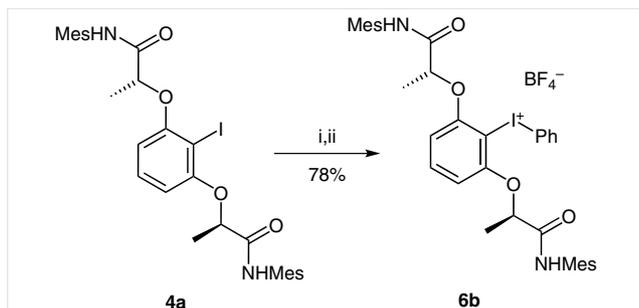
**Scheme 2** Direct oxidation and boron–iodine(III) exchange providing diaryliodonium salt **6b**. Reagents and conditions: i) MCPBA (1.8 equiv),  $\text{BF}_3 \cdot \text{OEt}_2$  (2.5 equiv),  $\text{CH}_2\text{Cl}_2$ , 0 °C, 2 h; ii)  $\text{PhB}(\text{OH})_2$ , r.t., 4 h, 78%.
