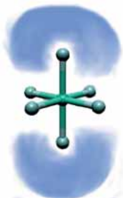
Figure 1.3: An idealised system \text{Gd(III)F}_6^{3-} , which has O_h symmetry will have no ZFS associated with it. However, if we distort the top and bottom atoms then the ground state degenerate energy levels will be split and ZFS begins to emerge.
