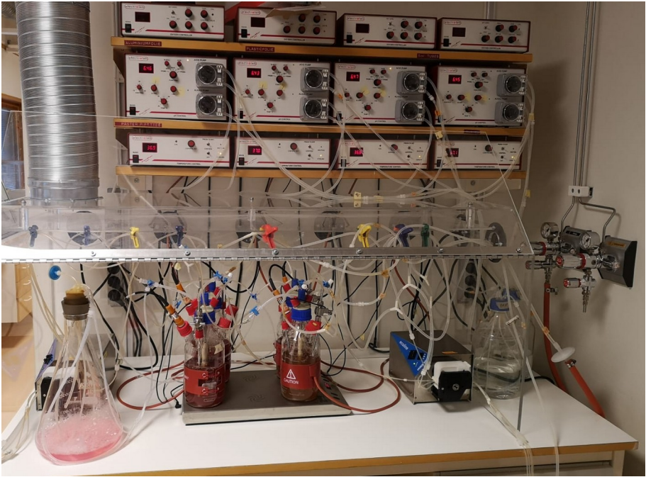
Figure 8. System of bioreactors to study long term cultures of polymicrobial communities including anaerobic conditions.
