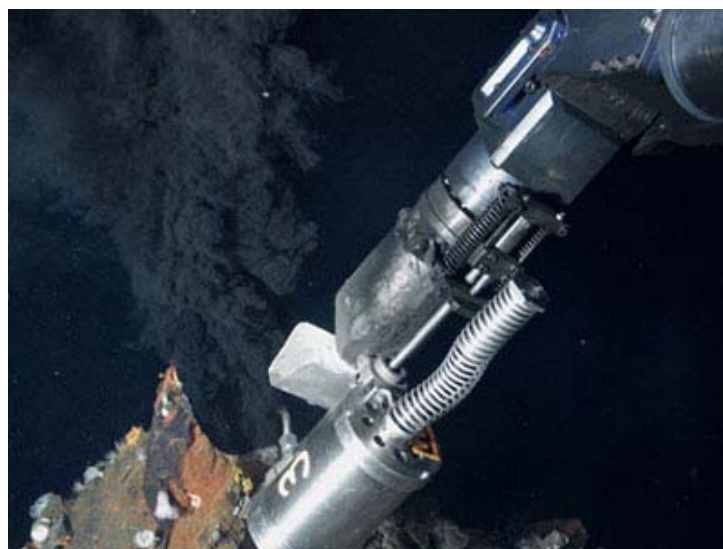
Figure 17: Sampling a black smoker. (Images © Ifremer / Serpentine 2007)
